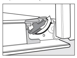
■ To release the locking clamps on the hinges turn them upwards as far as they will go until they are at an angle. See illustration.
